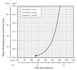
The AMCA Water Penetration Test provides a method for comparing various louver models and designs as to their efficiency in resisting the penetration of rainfall under specific laboratory test conditions. The beginning point of water penetration is defined as that velocity where the water penetration curve projects through .01 oz. of water (penetration) per sq. ft. of louver free area.
