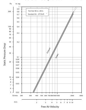
Model AFS-120 resistance to airflow (pressure drop) varies depending on louver application (air intake or air exhaust). Free area velocities (shown) are higher than average velocity through the overall louver size. See louver selection information.
