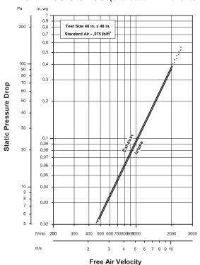
Model AFJ-120 resistance to airflow (pressure drop) varies depending on louver application (air intake or air exhaust). Free area velocities (shown) are higher than average velocity through the overall louver size. See louver selection information. (Tested to AMCA Figure 5.5 & 5.6)
