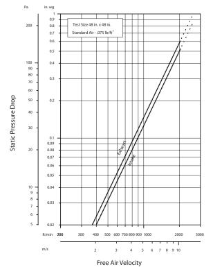
Model ESD-202 resistance to airflow (pressure drop) varies depending on louver application (air intake or air exhaust). Free area velocities (shown) are higher than average velocity through the overall louver size. See louver selection information.
