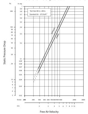
Model SES-202 resistance to airflow (pressure drop) varies depending on louver application (air intake or air exhaust). Free area velocities (shown) are higher than average velocity through the overall louver size. See louver selection information.
