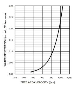
The AMCA Water Penetration Test provides a method for comparing various louver models and designs as to their efficiency in resisting the penetration of rainfall under specific laboratory test conditions. The point of zero water penetration is defined as that velocity where the water penetration curve projects through .01 oz of water penetration per sq. ft. of louver area. The beginning point of water penetration for SL-660 is 840 fpm free area velocity.
