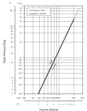
Model EDK-430 resistance to airflow (pressure drop) varies depending on louver application (air intake or air exhaust). Free area velocities (shown) are higher than average velocity through the overall louver size. See louver selection information.
