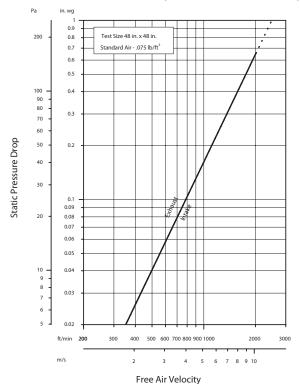
Model ESJ-602 resistance to airflow (pressure drop) varies depending on louver application (air intake or air exhaust). Free area velocities (shown) are higher than average velocity through the overall louver size. See louver selection information.
