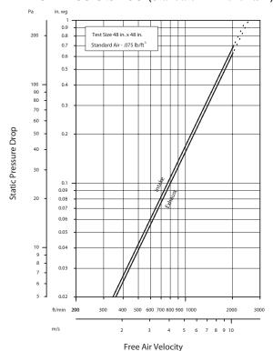
Model ESD-603 resistance to airflow (pressure drop) varies depending on louver application (air intake or air exhaust). Free area velocities (shown) are higher than average velocity through the overall louver size. See louver selection information.
