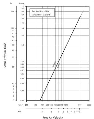
Model ESK-402 resistance to airflow (pressure drop) varies depending on louver application (air intake or air exhaust). Free area velocities (shown) are higher than average velocity through the overall louver size. See louver selection information.
