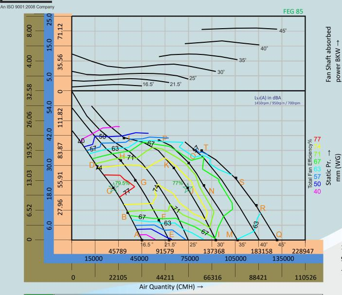
SOUND AIR Air Flow Private Limited certifies that the Vane Axial Flow Fan series AFPV4GVX shown herein are licensed to bear the AMCA seal. The ratings shown are based on tests and procedures performed in accordance with AMCA Publication 211 and AMCA Publication 311 and comply with the requirements of the AMCA Certified Ratings Program.
