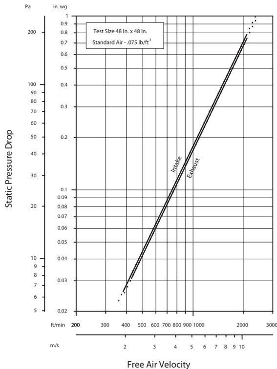
Model ESJ-401 resistance to airflow (pressure drop) varies depending on louver application (air intake or air exhaust). Free area velocities (shown) are higher than average velocity through the overall louver size. See louver selection information.
