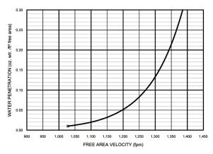
The AMCA Water Penetration Test provides a method for comparing various louver models and designs as to their efficiency in resisting the penetration of rainfall under specific laboratory test conditions. The point of zero water penetration is defined as that velocity where the water penetration curve projects through .01 oz of water penetration per sq. ft. of louver area. The beginning point of water penetration for AC-860 is 1,025 fpm free area velocity.
