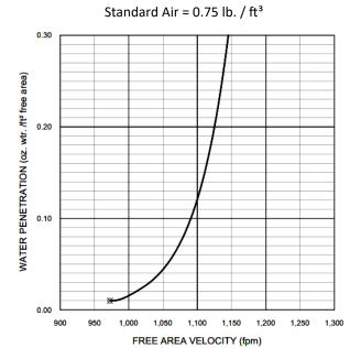
The AMCA Water Penetration Test provides a method for comparing various louver models and designs as to their efficiency in resisting the penetration of rainfall under specific laboratory test conditions. The point of zero water penetration is defined as that velocity where the water penetration curve projects through .01 oz of water penetration per sq. ft. of louver area. The beginning point of water penetration for DL-440 is 973 fpm free area velocity.
