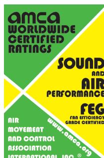
Certified FEGs are determined in accordance with AMCA 205-12 Energy Efficiency Classification for fans. In conjunction with AMCA 211-13 (Rev. 2015) Certified Ratings Program, Product Rating Manual for Fan Air Performance. This classification is based on fan peak (optimum) total efficiency for a given fan speed, fan size and application category. For the purpose of energy classification, the peak efficiency can be determined at a speed not higher than the maximum design speed of the fan.
