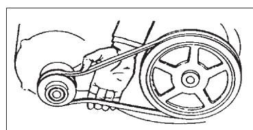
(Drawing 1) Belt tension bending of approx. 2-3 cm.
