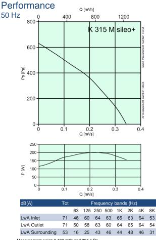
Measurement point: 0.180 m³/s and 394.1 Pa
