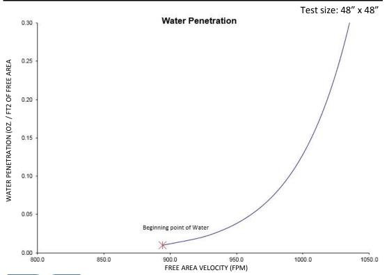
The AMCA Water Penetration Test provides a method for comparing various louver models and designs as to their efficiency in resisting the penetration of rainfall under specific laboratory test conditions. The beginning point of water penetration is defined as the velocity where the water penetration curve projects though 0.01 oz. of water (penetration) per sq. ft. of louver free area. \*The beginning point of water penetration for Model FA-40337 is 893 fpm free area velocity.
