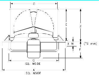
DIMENSIONAL DATA FAN в С E Fmax G Α SIZES IN IN IN IN mm IN mm IN mm mm mm mm  $16^{1}/$ 26 <sup>1</sup>/<sub>4</sub> 17<sup>1</sup>/2 14 <sup>7</sup>/<sub>8</sub> 16 <sup>3</sup>/<sub>8</sub> 416 15<sup>1</sup>/<sub>4</sub> 387 44 1118 31 <sup>1</sup>/ 34 <sup>1</sup>/ 19<sup>1</sup> 52 1321 19<sup>1</sup>/<sub>2</sub> 495
