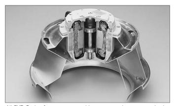
All FKD Series fans are powered by an external rotor motorized impeller. This design provides excellent heat dissipation even at low rpm. All of the FKD Series fans are 100% speed controllable through voltage reduction allowing for precision balancing of systems. FKD8XL through 18 are supplied standard with 115/1/60 motors. FKD18XL and FKD20 have a standard configuration of 230-460/3/60. For additional motor options please contact Fantech Technical Support at 1-800-747-1762.
