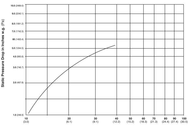
CFM (m³/min) Leakage per ft.² (m²) of Face Area Per AMCA Test #25587-E1
