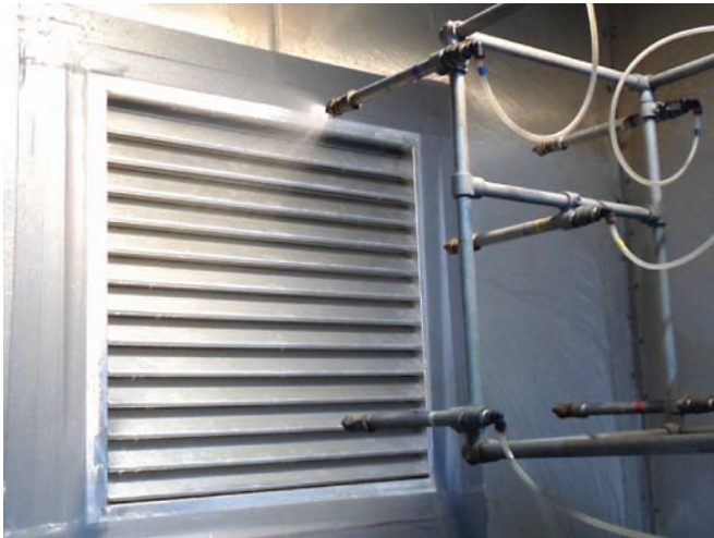
Wind Driven Rain Test conducted according to AMCA 500-L Figures 5.11
