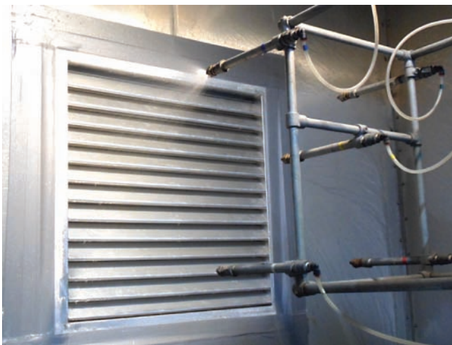
Wind Driven Rain Test conducted according to AMCA 500-L Figures 5.11
