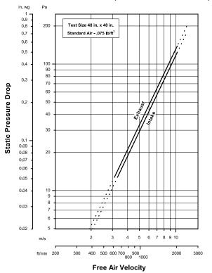
Model ESD-401SM resistance to airflow (pressure drop) varies depending on louver application (air intake or air exhaust). Free area velocities (shown) are higher than average velocity through the overall louver size. See louver selection information. (Test Figure 5.5-6.5)
