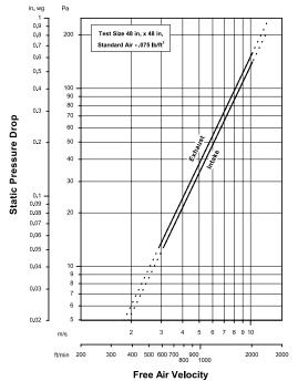
Model EAD-401SM resistance to airflow (pressure drop) varies depending on louver application (air intake or air exhaust). Free area velocities (shown) are higher than average velocity through the overall louver size. See louver selection information. (Test Figure 5.5-6.5)
