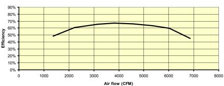
Impeller speed: 3550 rpm
