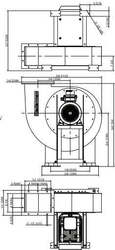
Duct inlet diameter 15 3/4 in Duct outlet diameter 15 3/4 in
