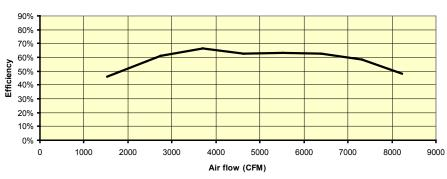
Impeller speed: 3540 rpm
