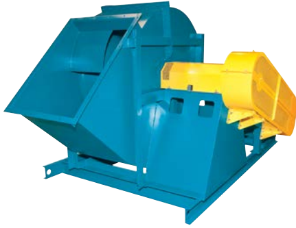
Arrangement 1 fan with optional unitary base, pie-shaped split housing, shaft and V-belt drive guard.
