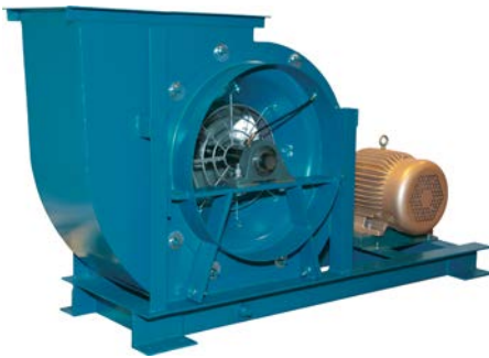
Arrangement 1 fan with optional unitary base, pie-shaped split housing, shaft and V-belt drive guard.
