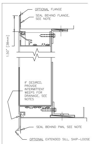
NOTE: SEALANT, BACKER ROD, NON-COMPRESSIBLE DEAD-LOAD SHIMS, SEPARATION OF DISSIMILAR MATERIALS AND SUBSTRATE ARE NOT BY LOUVER MANUFACTURER, SHIM AS NEEDED, PERIMETER SEALANT REQUIRED TO PASS ANSI/AMCA 550 HIGH VELOCITY WIND DRIVEN RAIN.
