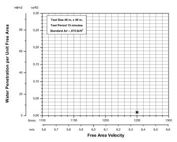
The AMCA Water Penetration Test provides a method for comparing various louver models and designs as to their efficiency in resisting the penetration of rainfall under specific laboratory test conditions. The beginning point of water penetration is defined as that velocity where the water penetration curve projects through 0.01 oz. of water (penetration) per sq. ft. of louver free area.
