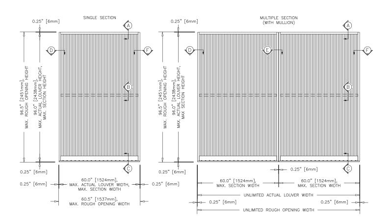
Minimum Rough Opening Size 12 in. W x 12 in. H Maximum Rough Opening Single Section Size 60 1/2 in. W x 96 1/2 in. H
