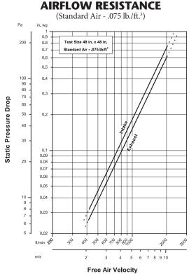
Louver Type SCV660MD resistance to airflow varies depending on louver application (air intake or air exhaust). Free area velocities (shown) are higher than the average velocity through the overall louver size. (Test Figure 5.5-6.5)
