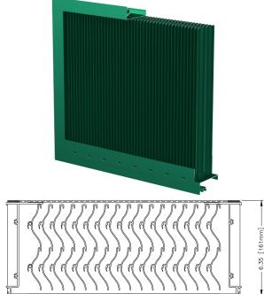
Approved. Louvers shall be 6-inches (152.4 mm) deep and assembled entirely from extruded aluminum components. Blades shall be 0.063-inch (1.60 mm) and frames shall be 0.095-inch (2.41 mm) thick aluminum, alloy 6063-T5. Blades shall be vertical, V-type with center hook and spaced 0.75-inches on center.
