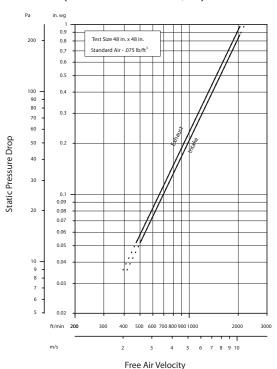
Louver Type SCH601MDE resistance to airflow varies depending on louver application (air intake or air exhaust). Free area velocities (shown) are higher than the average velocity through the overall louver size. (Test Figure 5.5-6.5)
