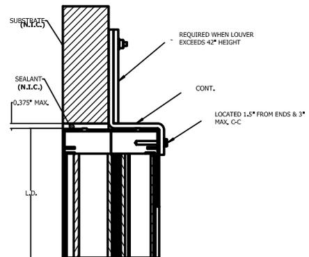
**ALT. CONT. ATTACHMENT ZEE INSTALLATION @ LOUVER HEAD/SILL**
