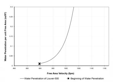
The beginning of water penetration defined as the velocity where the water penetration curves projects through .01 oz. of water (penetration) per ft² of louver free area. \*The beginning of water penetration per AMCA Publication 511 based on AMCA measured free area for model VTL-437 is 900.8 fpm.
