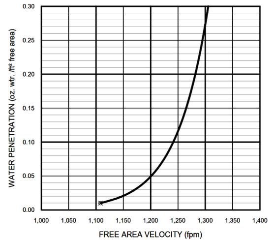
The AMCA Water Penetration Test provides a method for comparing various louver models and designs as to their efficiency in resisting the penetration of rainfall under specific laboratory test conditions. The point of zero water penetration is defined as that velocity where the water penetration curve projects through .01 oz of water penetration per sq. ft. of louver area. **The beginning point of water penetration for RSR-900 is 1,108 fpm free area velocity.**
