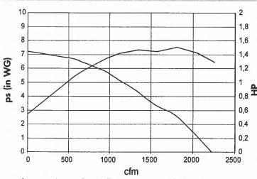
Performance shown is for installation type D: Ducted inlet, Ducted outlet. Performance ratings do not include the effects of appurtenance in the airstream. Performance measured at a speed of 3500 RPM and the effeciency of the motor.
