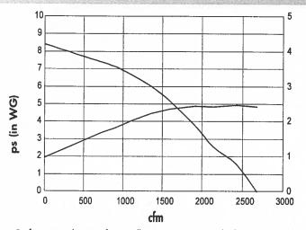
Performance shown is for installation type D: Ducted inlet, Ducted outlet. Performance ratings do not include the effects of appurtenance in the airstream. Performance measured at a speed of 3500 RPM and the effeciency of the motor.
