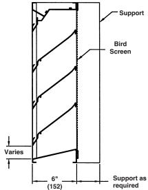
UL CLASSIFIED as a Wind Resistive Building Component in accordance with ASTM E330-02 for ±50 psf (2.39 kPA) windload. UL File No. R22052.
