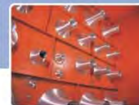
流量噴嘴 Multiple Nozzles for Flow Measurement
