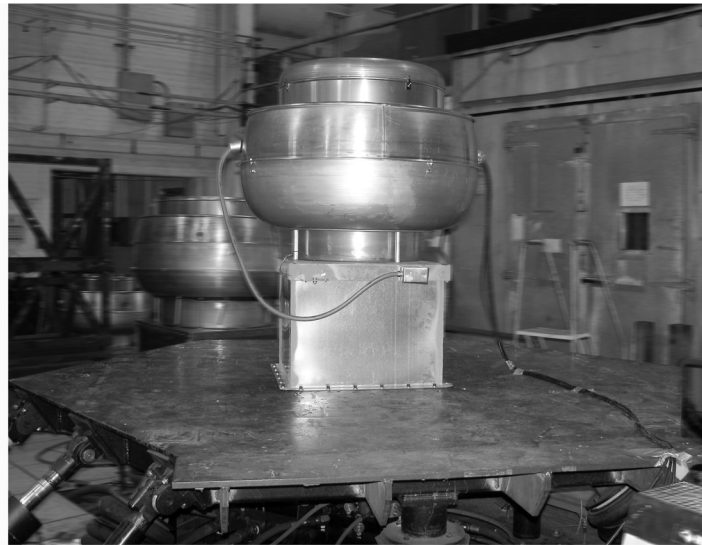
Seismic Simulation Test on Multi-Axis Shake Table
