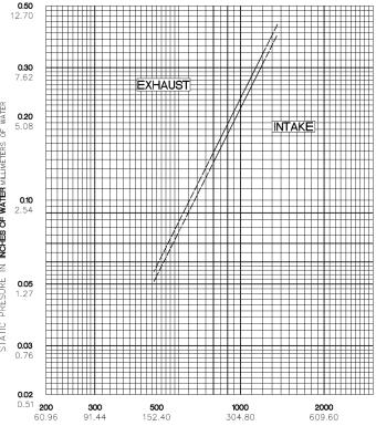
VELOCITY IN FEET AND METERS PER MINUTE THROUGH FREE AREA
