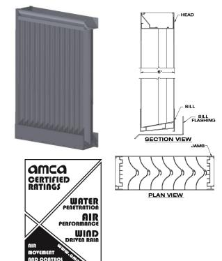
$\frac{\textbf{Discharge Coefficient}}{\textbf{Intake } C_d = \textbf{0.35 (Class 2)}}$
