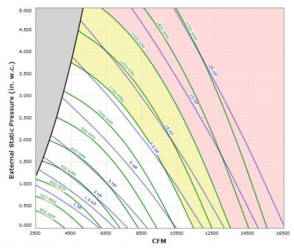
Max Sizeable RPM = 1300 RPM. Curve shown extended beyond this point for reference only.
