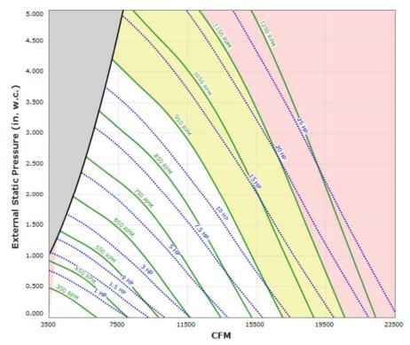
Max Sizeable RPM = 1150 RPM. Curve shown extended beyond this point for reference only.
