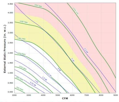
Max Sizeable RPM = 1700 RPM. Curve shown extended beyond this point for reference only.
