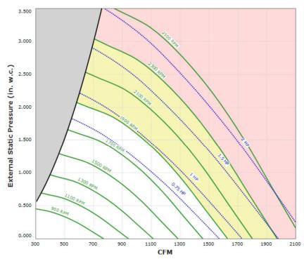
Max Sizeable RPM = 2300 RPM. Curve shown extended beyond this point for reference only.
