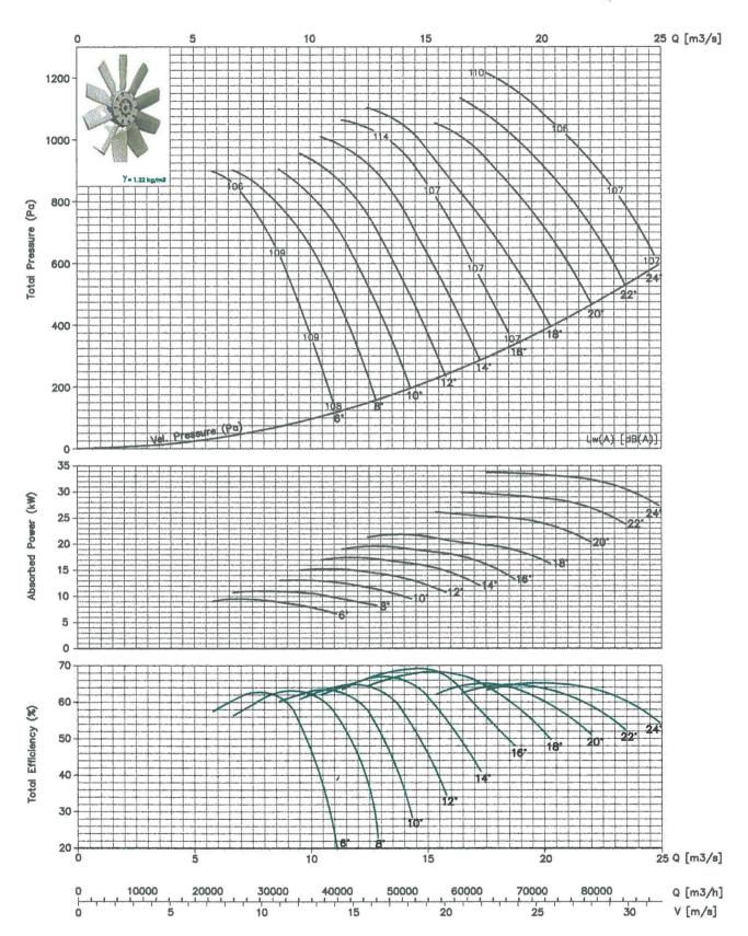
Performance shown is for installation type D - ducted inlet, ducted outlet. Performance ratings do not include the effects of appurtenances in the airstream.
