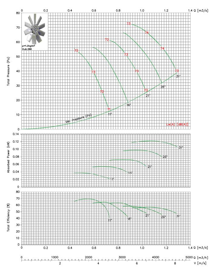
Performance shown is for installation type D - ducted inlet, ducted outlet. Performance ratings do not include the effects of appurtenances (accessories).
