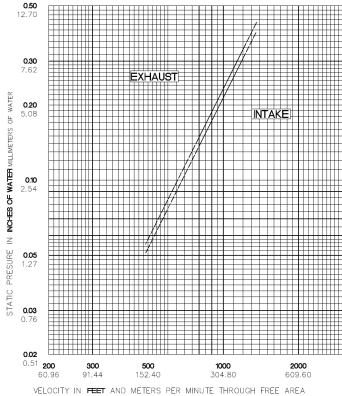
For a 48" x 48" sized louver Tested to AMCA Figure 5.5 Data corrected to standard air density
