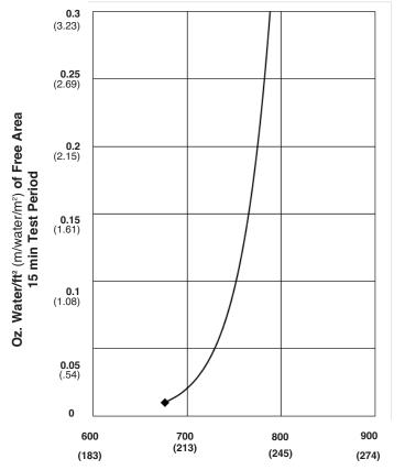
Test size 48" x 48" (1219 x 1219) Beginning point of water penetration at .01 oz./sq. ft. is 680 fpm (208 m/min.)
