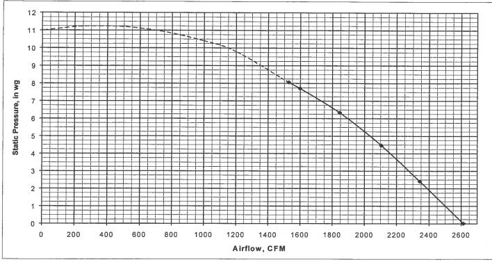
Performance shown is for installation type D – Ducted inlet, Ducted outlet. Performance ratings include the effects of inlet and outlet grilles in the airstream. Speed (RPM) shown is nominal. Performance is based on actual speed of test.
