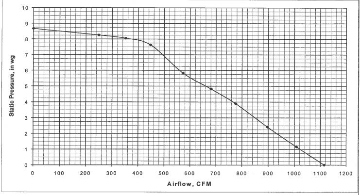
Performance shown is for installation type D – Ducted inlet, Ducted outlet. Performance ratings include the effects of inlet and outlet grilles in the airstream. Speed (RPM) shown is nominal. Performance is based on actual speed of test.
