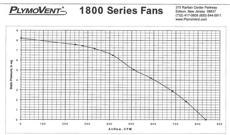
Performance shown is for installation type D – Ducted inlet, Ducted outlet. Performance ratings include the effects of inlet and outlet grilles in the airstream. Speed (RPM) shown is nominal. Performance is based on actual speed of test.
