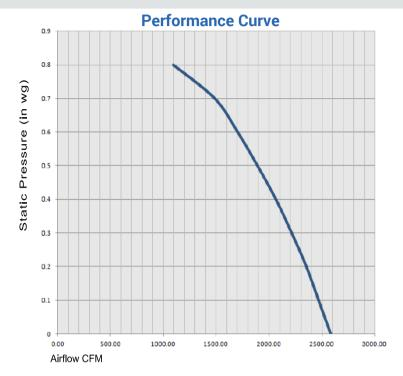
"Performance ratings do not include the effects of appurtenances(accessories). Performance certified is for installation type C: Ducted inlet, Unducted outlet per AMCA Standard 210. The Sound ratings shown are loudness values in fan sones at 1.5 m (5 ft) in a hemispherical free field calculated per AMCA International Standard 301. Values shown are for: Installation Type C: Ducted inlet, Unducted Outlet.
