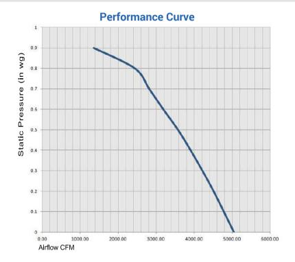
"Performance ratings do not include the effects of appurtenances(accessories). Performance certified is for installation type C: Ducted inlet, Unducted outlet per AMCA Standard 210. The Sound ratings shown are loudness values in fan sones at 1.5 m (5 ft) in a hemispherical free field calculated per AMCA International Standard 301. Values shown are for: Installation Type C: Ducted inlet, Unducted Outlet.
