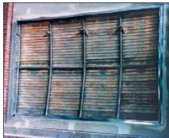
Photograph of actual UL 555 fire test conducted successfully at Underwriters Laboratories Inc., Northbrook Illinois.
