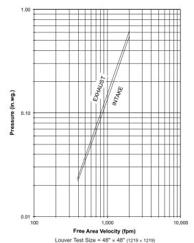
Pressure loss tested in accordance with Figure 5.5 of AMCA Standard 500-L.
